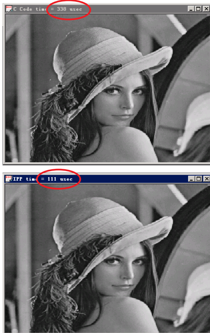
Figure 12: In this image resizing example (from 256x256 bits to 460x332 bits), the Intel® IPP-powered application ran in 111 msec vs. 338 msec for compiled C++ code (system configuration: Intel® Xeon, 2.9 GHz, 2 processors, 4 cores/processor, 2 threads/processor)
